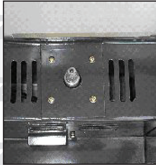
Gain access to saw shaft
